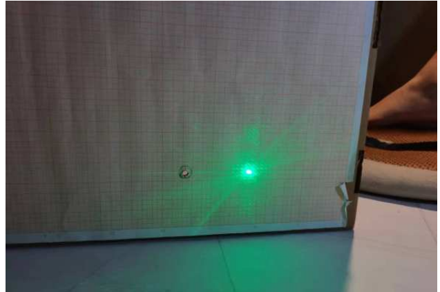
Figure 4.18 Diffraction pattern of OLED screen when laser is incident 30 degrees to the left
