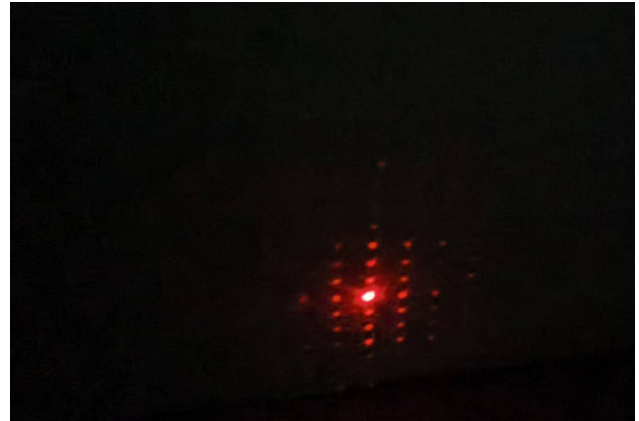
Figure 4.24 Diffraction pattern of LCD screen (using iPhone 7 plus as an example) when laser is incident at 60 degrees to the right
