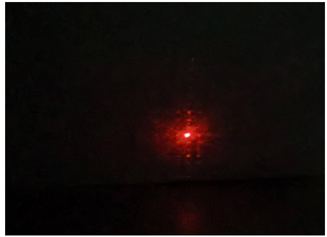
Figure 4.22 Diffraction pattern of LCD screen (using iPhone 7 plus as an example) when laser is incident at 30 degrees to the right
