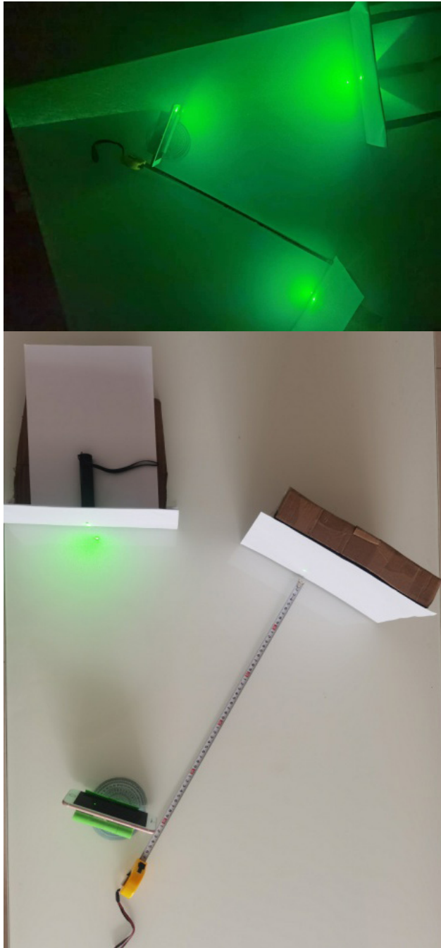
Figure 4.13 Diffraction experimental platform at an incidence angle of 30 degrees (in darkness and sunlight)
