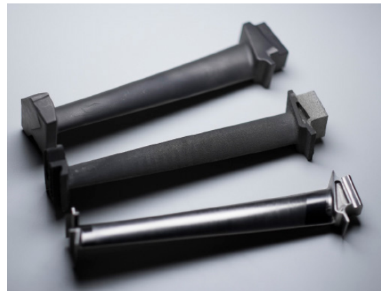
Fig.1 GE9X's TiAl low pressure turbine blade[8].
