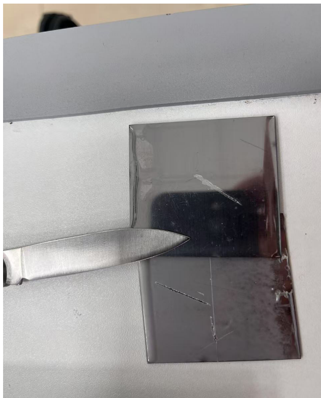
Picture 1 scars made by knife on coating
